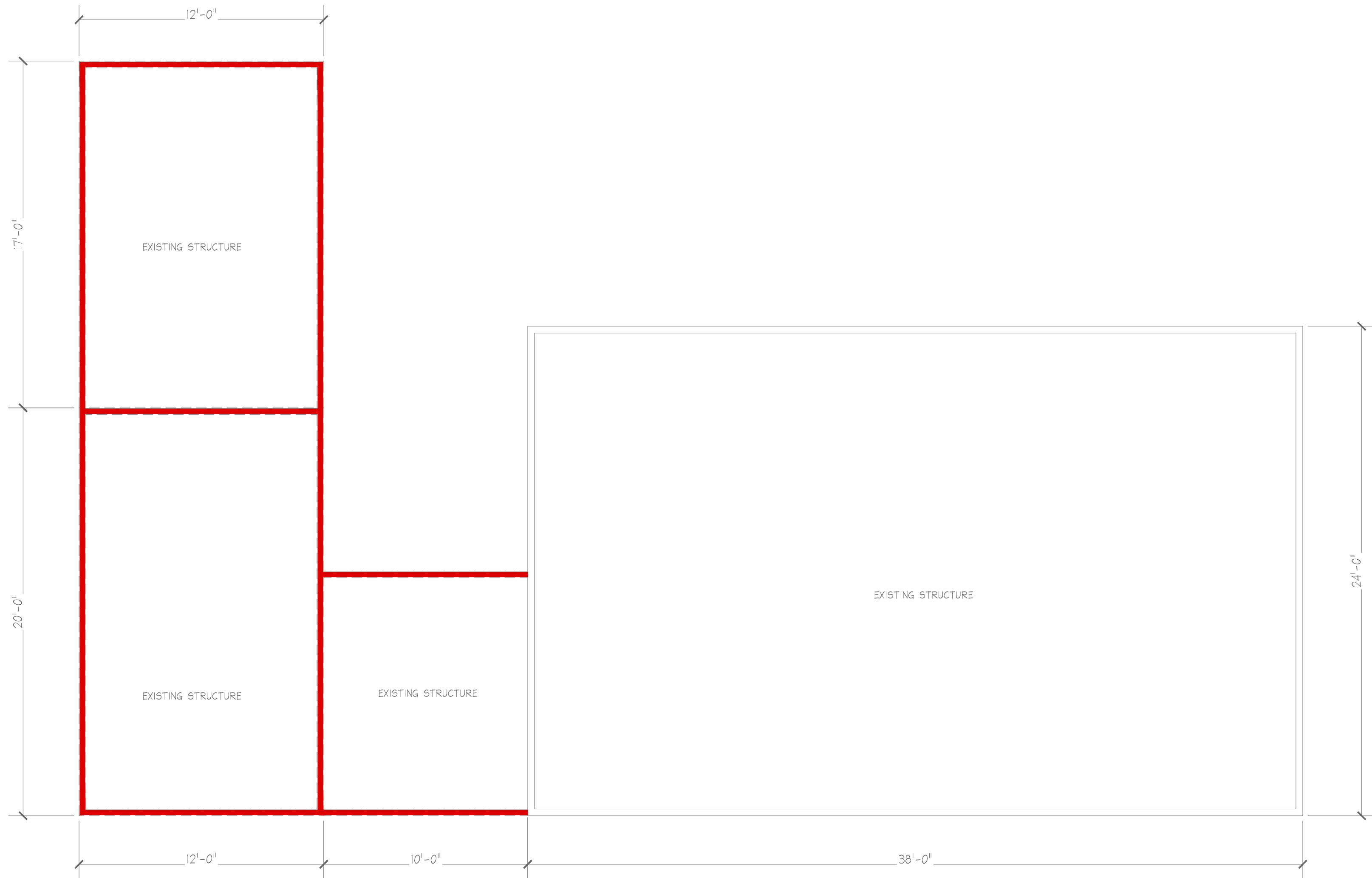
FIRST FLOOR DEMOLITION PLAN SCALE : 1/4"=1'-0" — - WALLS TO BE DEMOLISHED — - NEW WALL CONSTRUCTION
