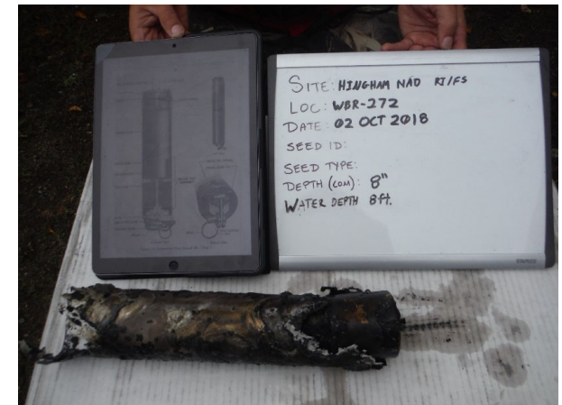
Photograph on this slide depicts the MDAS item (MK1 MOD1 Submarine Float Signal M69) recovered at the Weymouth Back River MRS
