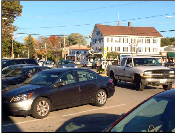
Figure 4-5: In Columbian Square, diagonal on-street parking reduces visibility and fast moving traffic causes senior pedestrians to feel unsafe. Photo by Nicholas Bulens
