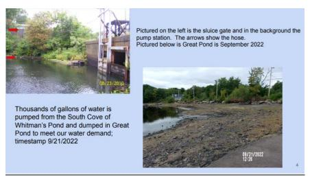
Weymouth has 5 wells, 3 surface systems. Water is treated at the Great Pond treatment facility. Whitman's Pond is only to be used as an emergency backup. There is a draft protocol for the operation of the sluice gate at South Cove of Whitman's Pond but not an approved one. She explained the procedure to pump from the South Cove. The height of Great Point triggers the water restrictions under drought situation.
