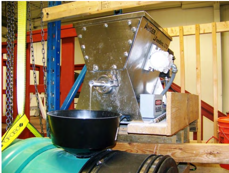
Figure 8 Sediment Addition Point
