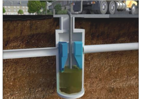
Fig.2 Maintenance is performed with a vacuum truck.
