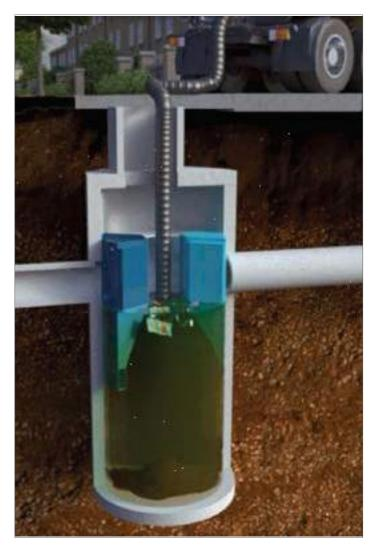
*Fig.4 Floatables are removed with a vactor hose (First Defense model FD-4, shown).*
