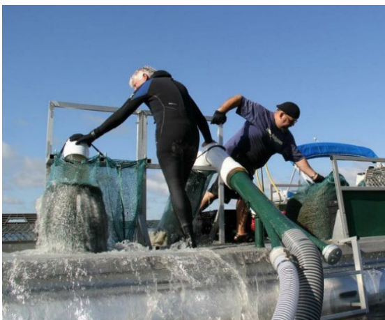
DASH operations are able to pump harvested weeds directly into mesh bags on deck, reducing the amount of fragmentation in the water.
