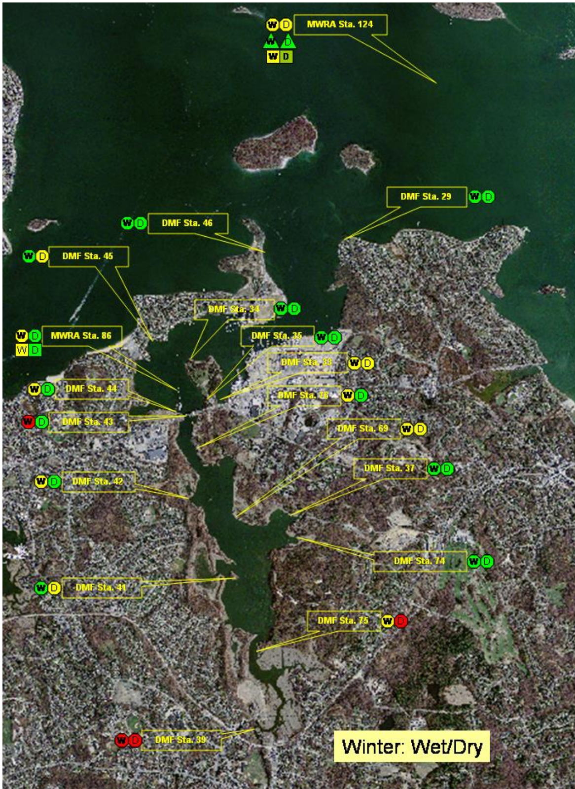
Figure 6-4. Winter Fecal Coliform Exceedances in Weymouth Back River (1992-2008). Exceedances of Massachusetts water quality standards for Fecal Coliform bacteria during winter (November-April) sampling events (Massachusetts Dept. of Marine Fisheries). Red
