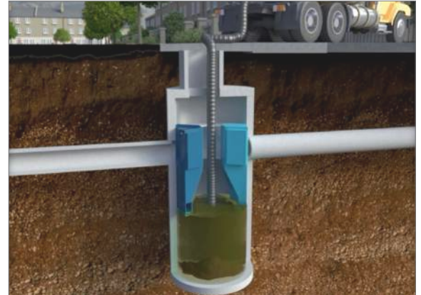
Fig.2 Maintenance is performed with a vector truck.
