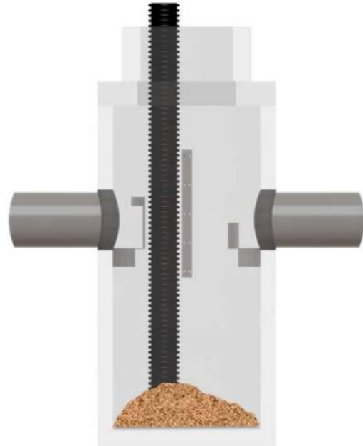
Insert Vacuum Hose On the Inlet Side of the Oil/Floatables Skimmer and Vacuum Out All Trash, Sediment and Standing Water.
