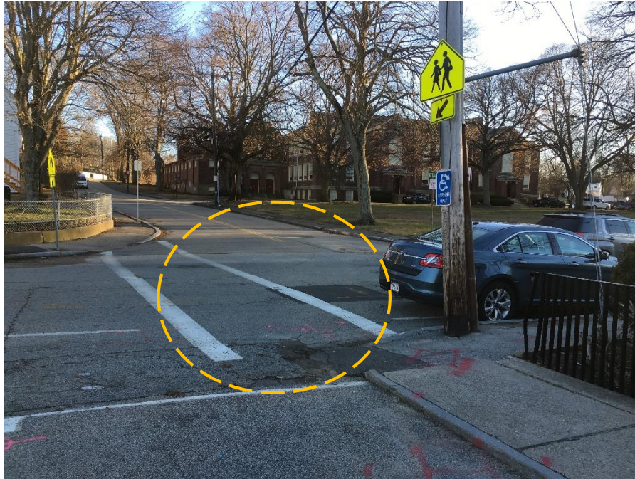
Figure 29: Corner of the Library's driveway at Broad Street. On-street parking obstructs visibility of pedestrians in crosswalk and creates "blind" turning conditions for vehicles exiting driveway.
